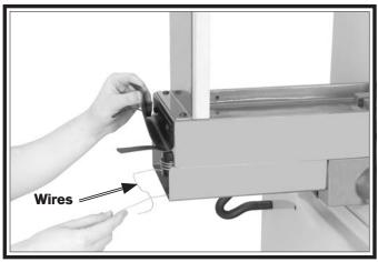
Figure 13. Neoprene shipping seat wires.
